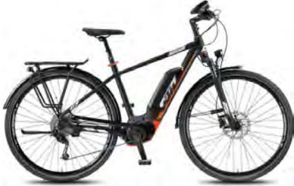
KTM Macina Fun Shimano 9-Gang Deore Bosch Performance CX 85 Nm, 500Wh Akku
